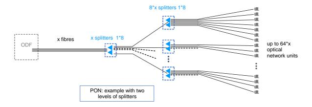
PON operators need to achieve a balance between optimising investment costs (optimising occupancy on the branches, but with a need for regular work to be performed at the points of flexibility where the splitters are located) and optimising operating costs (limiting the amount of work done at the flexibility points, which implies a lower rate of occupancy on the branches).
