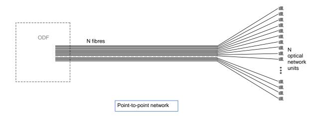
In addition, the installation of optical distributors can require a substantial investment as there are, in principle, as many optical fibres arriving at this concentration point as there are households located in the ODF's service area (several thousand). Although the optical fibre takes much less space that copper telephone lines, the ODFs can nevertheless occupy a sizeable area.
